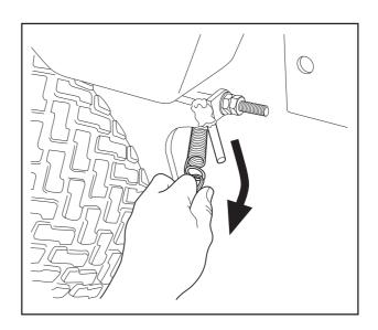
6. Place a foot on the front edge of the cutting unit near the wheel and raise the front edge of the unit to make it easier to remove the lift strut. Engage the strut in the holder.
